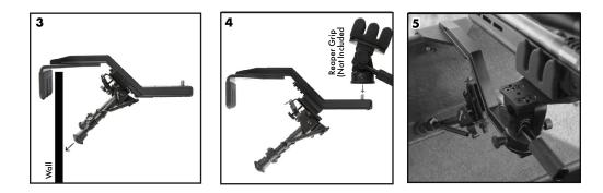
blind designs, is the Picatinny rail section. It is important to attach the bipod on the correct section of rail, as well as make sure the bipod legs are angled out and extended until the Ambush Rail is parallel to the floor of the blind. (figure 3) Extending or reducing the length of the bipod legs ensures a secure attachment of the Ambush to the blind at the proper angle.
